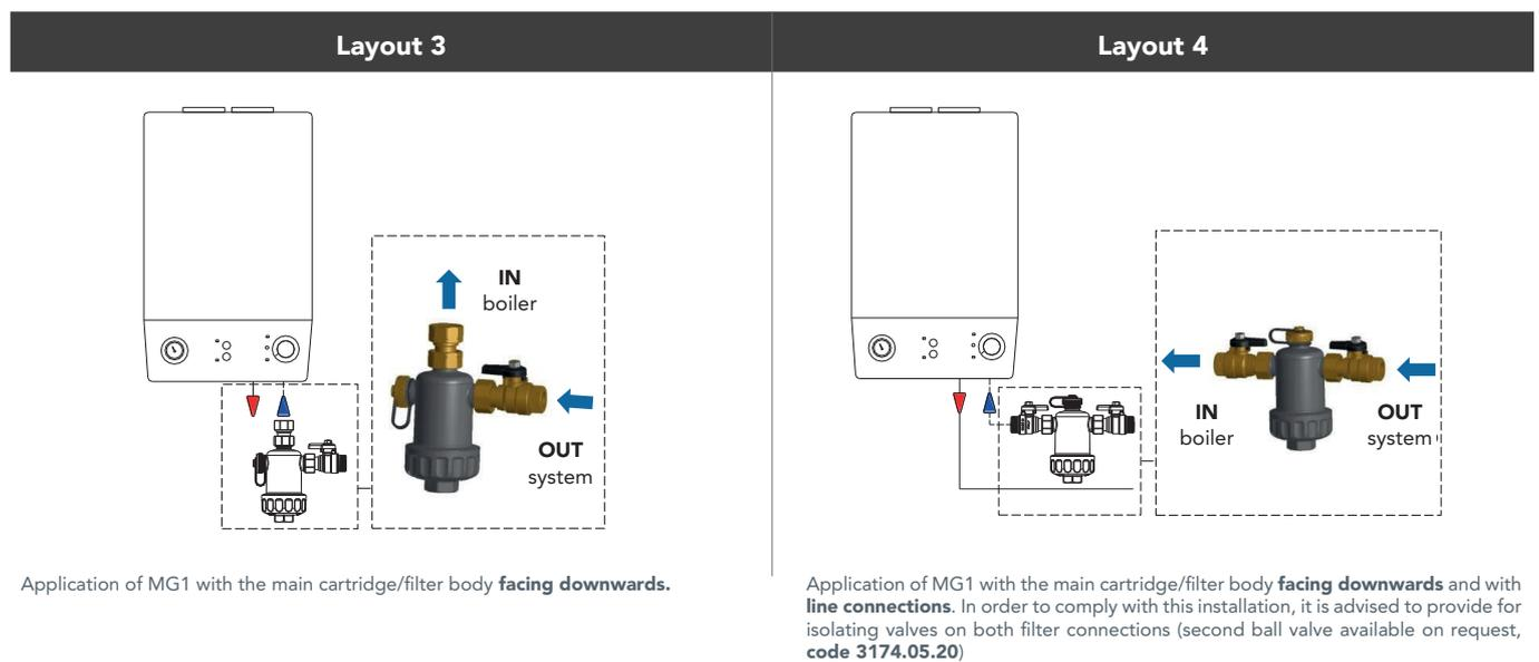
In order to allow the implementation of these installation configurations, it is sufficient to invert the position of the boiler connection swivel fitting and the ball valve (specifically in "Layout 2" and "Layout 4" also the drain cap) and rotate the filter by 90°.
