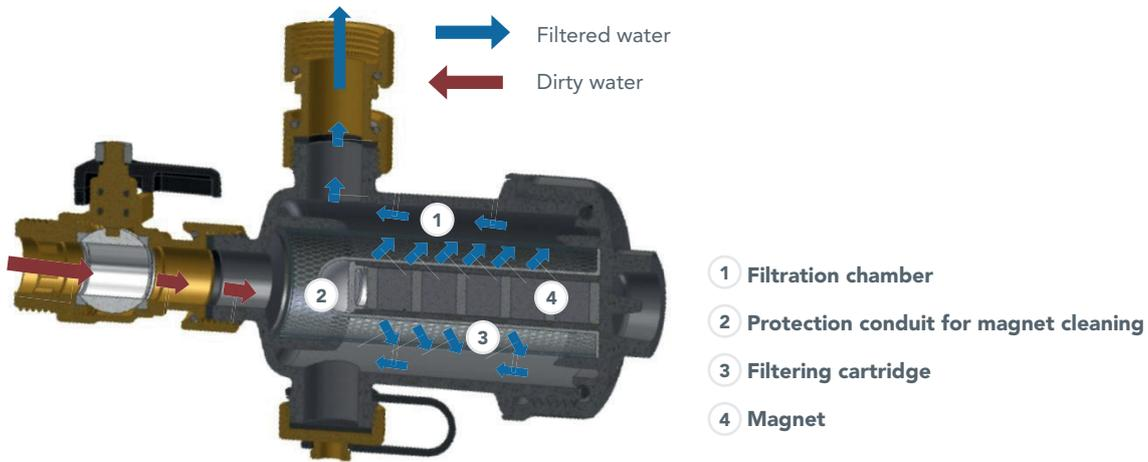
By going through a set course, the fluid is forced to cross the mesh of the cartridge and enter the filtration chamber.
